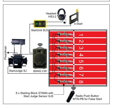
The start system BANG CW can also be implemented into an athletic false start system. When the impulse device e-Start is triggered the BANG CW and the speakers of the false start system StartJudge SJ imitate a gun shot. If the starter triggers the e-Start again within 5 seconds the speakers release a false start sound. With the radio push button WTN-PB the recaller can activate a false start signal (no start impulse).
