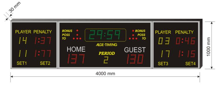
This Score Board consists of 3 modules which are mounted to metal frame.
